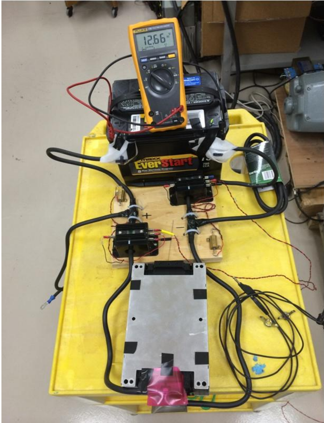
Figure 7.2. Balanced parallel connection Hybrid ESS.
